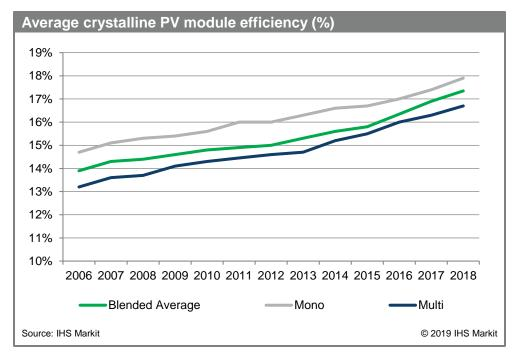
The trend of using monocrystalline cell technology is an increasingly important factor, when it comes to increasing average efficiency. In particular, PERC cells are becoming a mainstream technology, accounting for half of global cell production in 2019, compared to just 14 percent in 2016.
